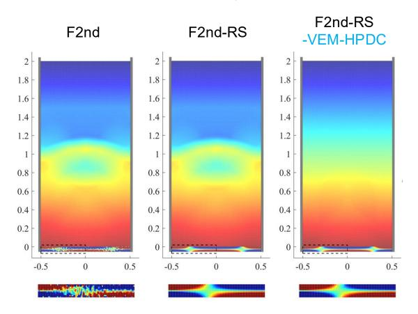
Reduces noises in both fluid and structure fields
